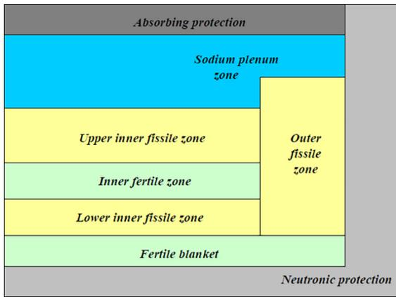
Fig. 2. Heterogeneous core Layout of the CFV Core.
