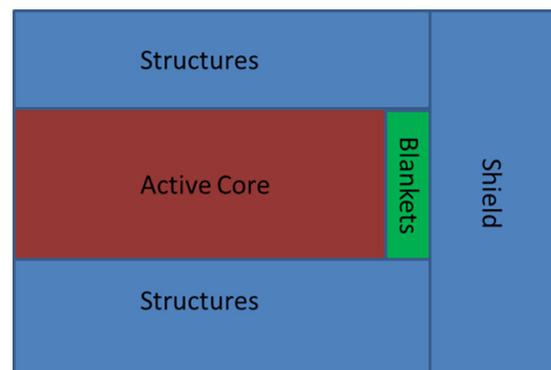
Fig. 1. Homogeneous core layout of the SFR V2b.
