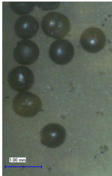
Fig. 4. Am-bearing blanket pellets fabricated for the MARINE irradiation.
