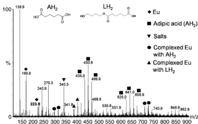
**Figure 8:** ESI-MS spectrum in positive mode of Eu in solution with HDPs from  $\gamma$ -PURE:  $[\text{Eu}] = 10^{-6} \text{ mol} \cdot \text{kg}_w^{-1}$ ,  $\text{pH} = 9.4$ ; HDPs are released after the leaching of the polymer in ASCPW solution for one month at  $60^\circ\text{C}$ . The signal attributions in Table 4 were done by ESI-MS-MS, and correspond to Eu complexed by adipic acid ( $\text{AH}_2$ ) and a soft segment oligomer ( $\text{LH}_2$ ).
