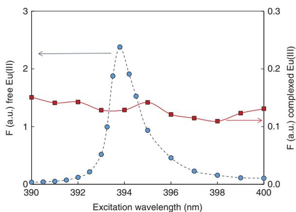
**Figure 3:** Excitation spectra of  $[\text{Eu}] = 10^{-6}\text{ mol}\cdot\text{kg}_w^{-1}$  at pH 4.1 (blue circles, dashed line), and complexed by HDPs ( $1.6\text{ mol}\cdot\text{kg}_w^{-1}$ ) from  $\gamma$ -PURE in SACPW solution (red squares, solid line):  $D = 10\ \mu\text{m}$ ,  $W = 300\ \mu\text{s}$ , 2000 accumulations.
