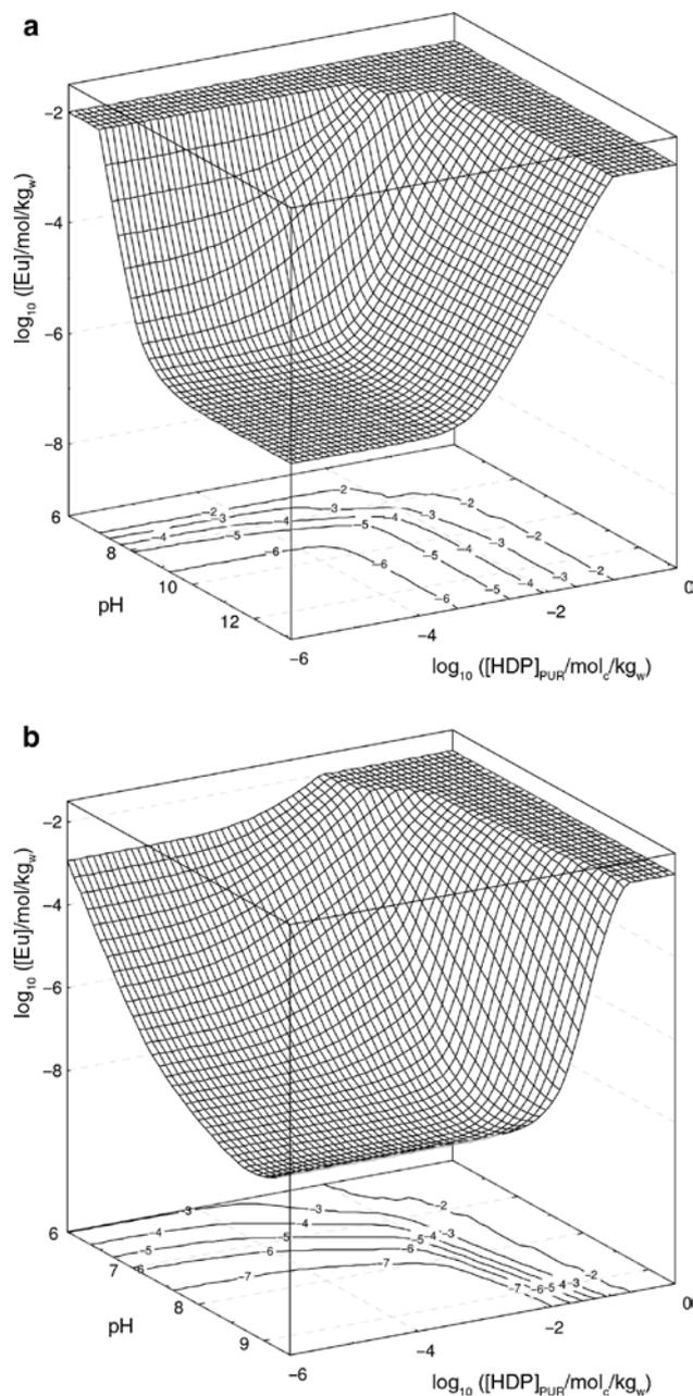
**Figure 9:** The solubility enhancement of  $10.01 \text{ mol} \cdot \text{kg}_w^{-1} \text{ Eu}(\text{OH})_3(\text{am})$  by  $\gamma$ -PURE HDP and comparison with the solubility of  $\text{EuOHCO}_3(\text{cr})$  at atmospheric  $\text{CO}_2(\text{g})$  pressure.
