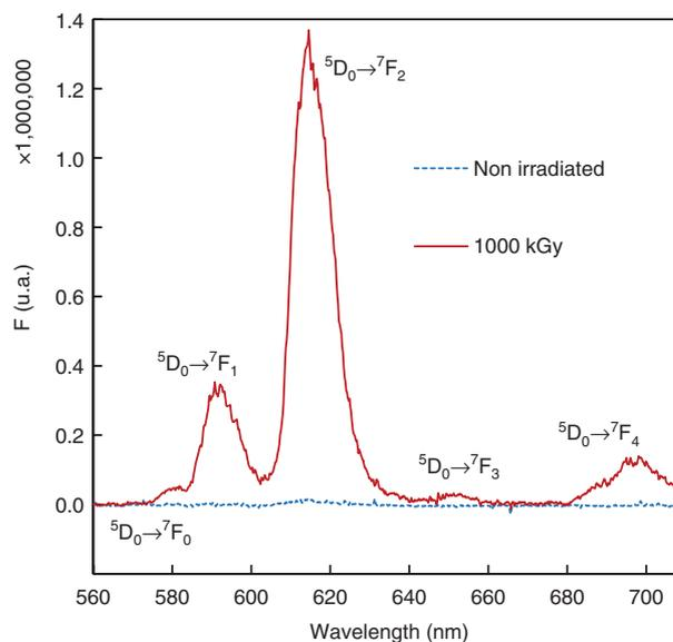
**Figure 2:** Luminescence spectra of Eu(III) in solution with HDPs from non-irradiated PURE (dotted line) and  $\gamma$ -PURE (plain line) in SACPW:  $[\text{Eu}] = 10^{-6} \text{ mol} \cdot \text{kg}^{-1}$ ;  $D = 10 \mu\text{s}$ ,  $W = 300 \mu\text{s}$ ,  $\lambda_{\text{exc}} = 393.8 \text{ nm}$ . HDPs are released after the leaching of the polymer in the SACPW solution for one month at 60 °C. HDPs were diluted by two to obtain these spectra.
