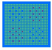
Figure 4: (Color online) Radial view of the TRIPOLI-4  $^{\textcircled{R}}$  model of the IPEN/MB-01 core.
