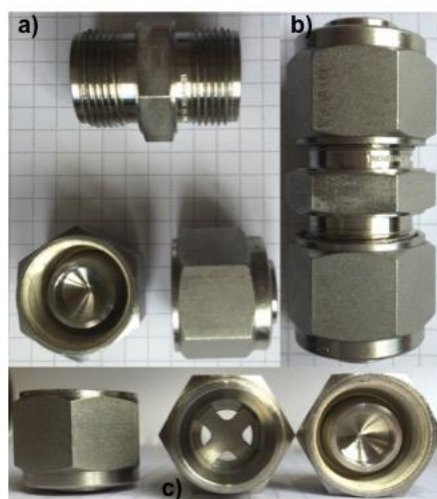
Figure 1. Open Swagelok connector (a), closed experimental capsule (b), stainless steel separator (c).
