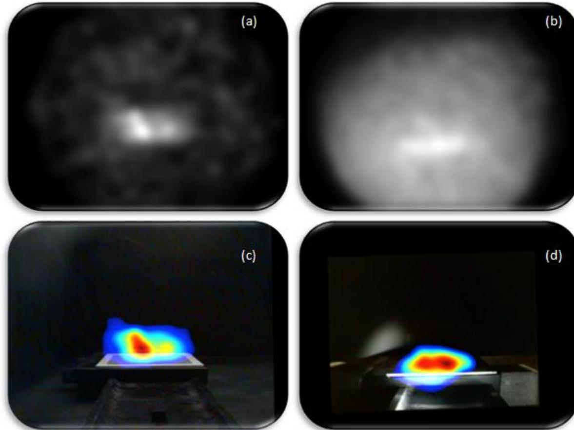
(a, b) Raw Alpha/UV Images with FFT filtering (a : Solar Blind, b : Low-Noise S20)
