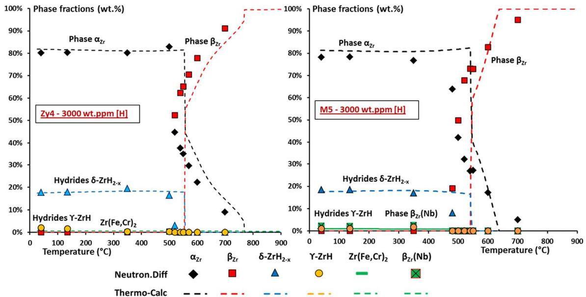
Figure 1: Evolution of phase weight fractions as a function of temperature obtained by neutron diffraction (symbol) *in situ* during step-cooling from 700°C and thermodynamic calculations (dotted curves) for Zircaloy-4 (left) and M5 (right) containing about 3000 wt.ppm of hydrogen
