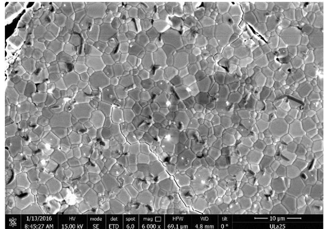
Fig. 1. SEM picture of the U<sub>0.75</sub>La<sub>0.25</sub>O<sub>2-x</sub> sintered pellet
