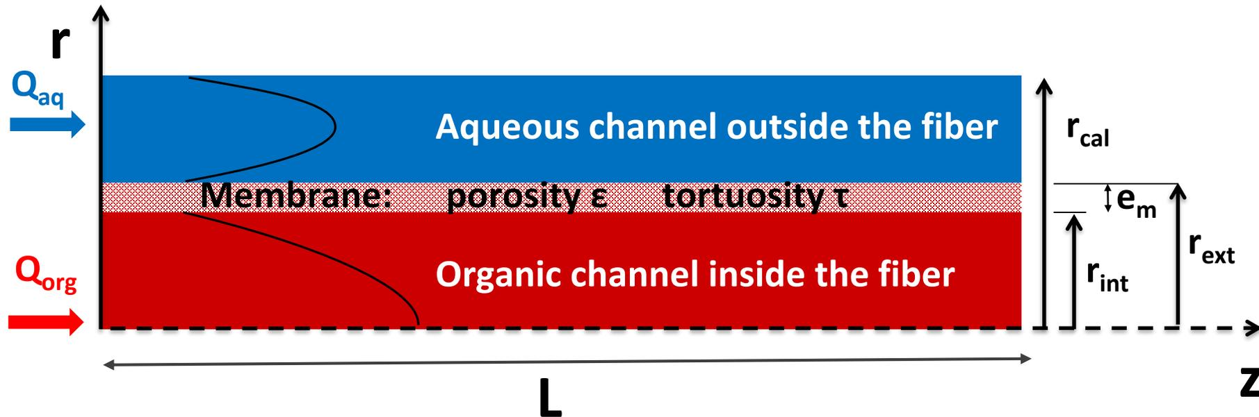
Laminar flow ( $Re < 1$ )  $\rightarrow$  axisymmetric Hagen-Poiseuille flow
