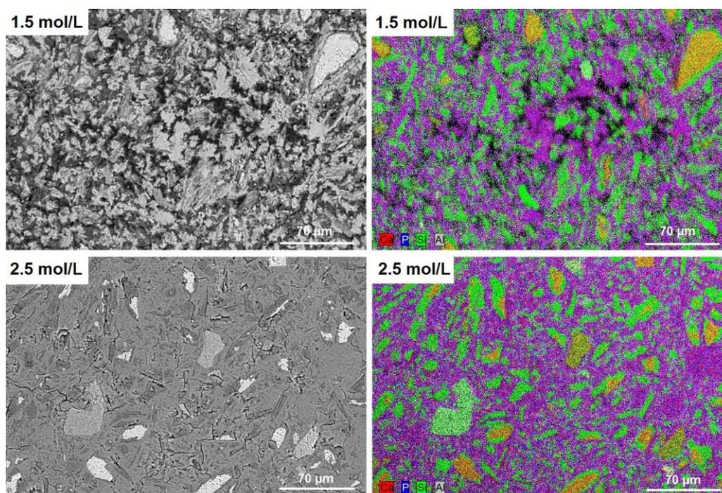
**Figure 10. Comparison of the microstructure of 28 d-old cement pastes prepared with a mixing solution containing 1.5 or 2.5 mol/L of Al<sup>3+</sup> ([B] = 0 mol/L): BSE images (left) and elemental mapping (right).**
