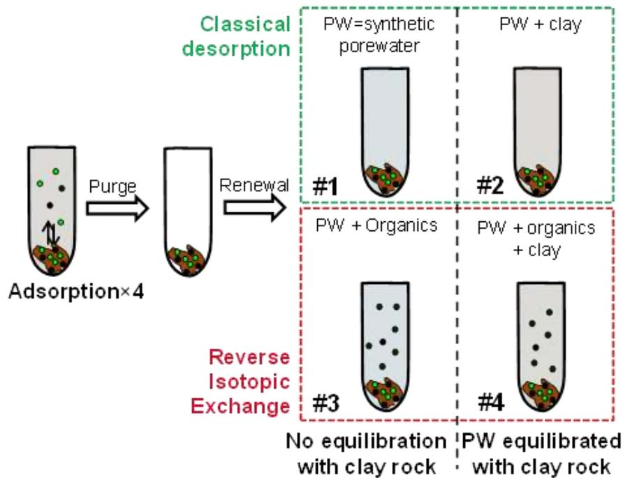
Figure 2. Scheme of the desorption protocols #1 to #4, with various renewal solutions.  $^{12}\text{C}$ - and  $^{14}\text{C}$ -organics are represented in black/green points respectively. Synthetic and clay-equilibrated pore waters are represented in blue and brown respectively.
