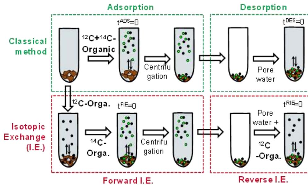
Figure 1. Scheme of adsorption and desorption experimental setup. Comparison of classical batch method (top) and isotopic exchange (bottom).  $^{12}\text{C}$ - and  $^{14}\text{C}$ -organics are represented by black and green dots respectively.
