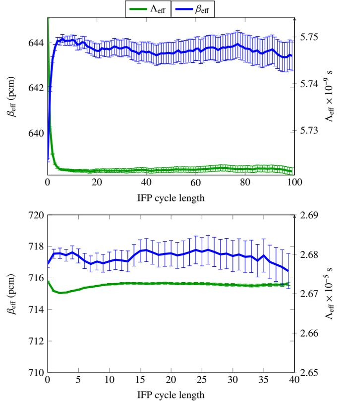
Figure 6: Top. The kinetics parameters  $\beta_{\text{eff}}$  and  $\Lambda_{\text{eff}}$  as a function of the IFP cycle length  $M$  for the GODIVA configuration of the Rossi alpha validation suite. Error bars represent statistical uncertainty at  $1\sigma$ . Bottom. The kinetics parameters  $\beta_{\text{eff}}$  and  $\Lambda_{\text{eff}}$  as a function of the IFP cycle length  $M$  for the N4 PWR reactor. Error bars represent statistical uncertainty at  $1\sigma$ .
