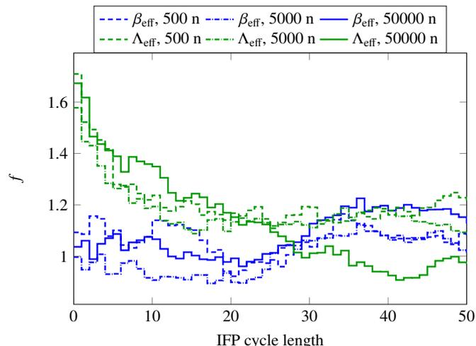
Figure 8: Inter-cycle correlations on  $\beta_{\text{eff}}$  and  $\Lambda_{\text{eff}}$  for the  $N4$  PWR reactor. The factor  $f = \hat{\sigma}/\hat{\sigma}_a$  is plotted as a function of the IFP cycle length  $M$ . Large deviations from  $f \approx 1$  imply strong inter-cycle correlations.
