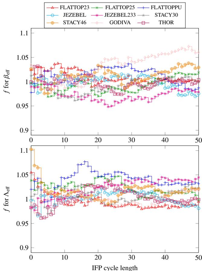
Figure 7: Inter-cycle correlations on  $\beta_{\text{eff}}$  and  $\Lambda_{\text{eff}}$  for some of the reactor configurations in the Rossi alpha validation suite. The factor  $f = \hat{\sigma}/\hat{\sigma}_a$  is plotted as a function of the IFP cycle length  $M$ . Large deviations from  $f \approx 1$  imply strong inter-cycle correlations.
