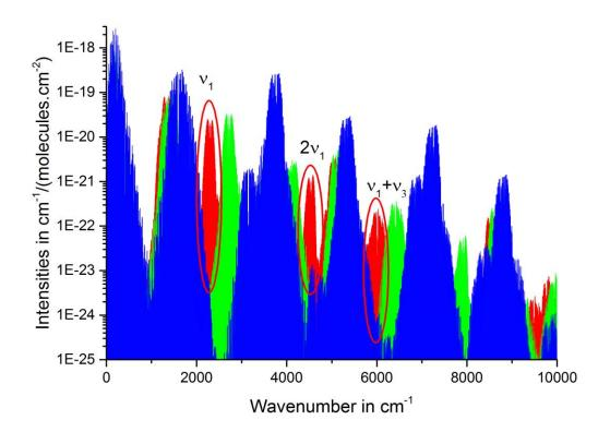
Figure 2: theoretical absorption spectra of 10 mbar pressure water stable isotopes  $\rm H_2^{16}O$ ,  $\rm H_2^{17}O$ ,  $\rm H_2^{18}$  and HDO (blue), with natural isotopy. The red line is the absorption spectra of  $10^{-6}$  molar fraction of HTO [10].
