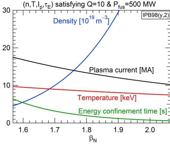
**Figure 2.** Normalized density, temperature, plasma current and energy confinement time associated to the  $(R, B)$  couples of figure 1. The dashed horizontal lines correspond to the interval of temperatures where  $\langle \sigma v \rangle$  scales like  $T^2$ .
