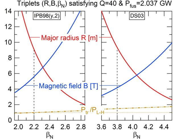
**Figure 5.** Same as figure 1 for DEMO specifications (here,  $P_{tr}$  is calculated by assuming that 66% of the heating source is radiated, cf. text). Both IPB98(y,2) and DS03 scaling laws are considered.
