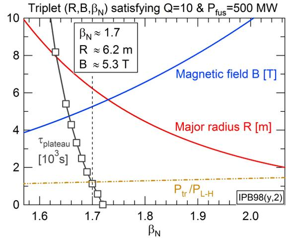
**Figure 1.** Values of  $R$  and  $B$  as a function of  $\beta_N$  which fulfill both equations (8) and (15) when using the IPB98(y,2) scaling law. The solution at  $\beta_N \approx 1.7$  is close to the ITER specifications  $R_{ITER} = 6.2 \text{ m}$ ,  $B_{ITER} = 5.3 \text{ T}$ . The plasma is supposed to be in H-mode if the ratio  $P_{tr}/P_{L-H}$  (see text for definitions) is above unity. The plateau duration  $\tau_{plateau}$  is discussed in section 3.3.
