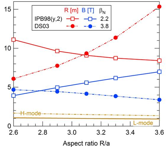
**Figure 6.**  $R$  (red) and  $B$  (blue) solutions for DEMO when varying the aspect ratio  $R/a$  at fixed  $\beta_N$ :  $\beta_N = 2.2$  for the IPB98(y,2) scaling law (plain lines), and  $\beta_N = 3.8$  for the DS03 one (dashed lines). The ratio  $P_{tr}/P_{L-H}$  is also plotted, in the same way as for figure 5.
