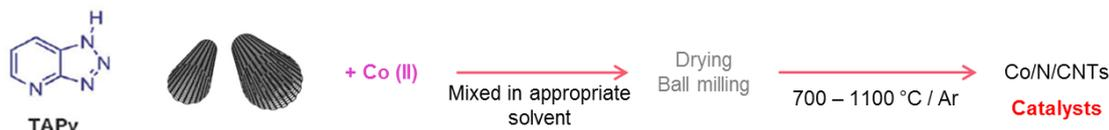
Scheme 1: Method for preparing N-functionalized CNTs catalysts
