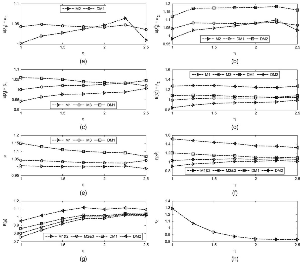
Fig. 4. Ratios of theoretical to numerical simulation results for  $\beta = 0.02$  and various  $\eta$ : (a)  $\alpha_1$ ; (b)  $\alpha_2$ ; (c)  $\beta_1$ ; (d)  $\beta_2$ ; (e)  $p$ ; (f)  $E[d^2]$ ; (g)  $E[\mu]$ ; and (h)  $\tau_c = 1/\mu_\gamma$ .
