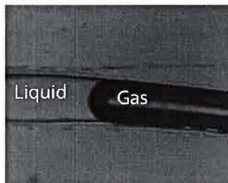
FIGURE 3: Optical image of a fluid front in a 300 microns rolled up system.
