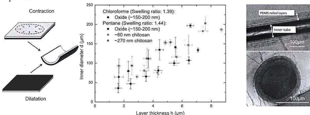
FIGURE 1: *Left* : Two types of rolling of a bilayer systems. Either the top layer shrinks (top) or the bottom layer is swollen by a solvent (bottom). The flat position is not equilibrium anymore so that a spontaneous curvature occurs. *Center* : Inner diameter as a function of film thickness for different types of capping and solvents in the case of the swelled PDMS process. *Right* : Optical images of rolled systems embedded in PDMS, side and front view.
