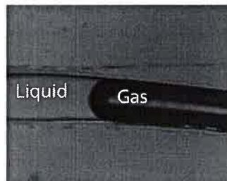
FIGURE 3: Optical image of a fluid front in a 300 microns rolled up system.
