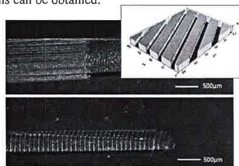
FIGURE 2: *Inset* : Pattern of a PDMS film before rolling. The grooves depth is 11.2 microns. *Main* : Patterned rolled systems with different rolling directions. *Top* : Grooves parallel to axis.
