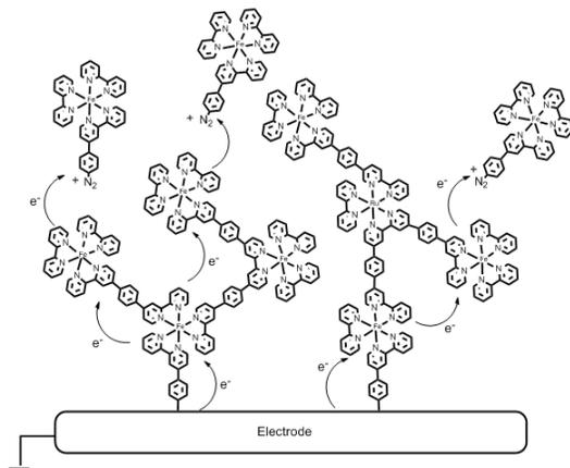
Scheme 1. Scheme of an electrografting of a diazonium salt of TBPFdiazonium on a gold electrode.
