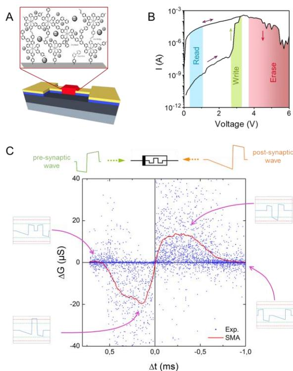
**Figure 1:** A) Planar structure of the organic memristor and schematic of the electro-grafted thin film of redox complexes. B) Unipolar switching behavior of single memristor. C) Cumulative STDP property of single organic memristor during ~4300 sequentially-applied voltage pulses with random time-delay of pre-/post-synaptic input.
