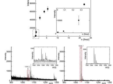
Figure 3. Average MS signal intensity as a function of the amount n (n from 22 femtomoles to 17 attomoles) of Angiotensin II deposited on the MALDI plate by the microfluidic platform deposit.
