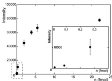
Figure 3. Average MS signal intensity as a function of the amount  $n$  ( $n$  from 22 femtomoles to 17 attomoles) of Angiotensin II deposited on the MALDI plate by the microfluidic platform deposit.
