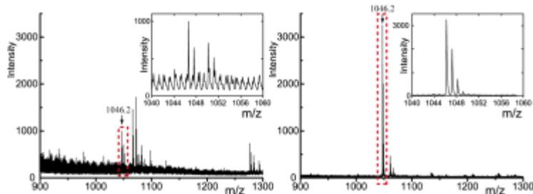
Figure 4. MALDI spectra of a 100 attomoles solution of Angiotensin II. *Left.* Microfluidic platform deposit. *Right.* Microfluidic platform multi-spotting deposit. Inserts: zoom on Angiotensin II peaks.
