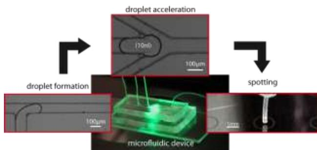
Figure 1. Principle of the droplet formation and MALDI deposition
