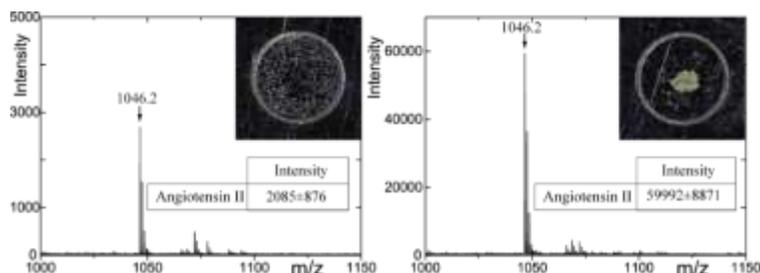
Figure 2. MALDI spectra. *Left.* Standard pipette deposit. *Right.* Microfluidic platform deposit. Inserts: Dried mixture of peptide/matrix before laser desorption.
