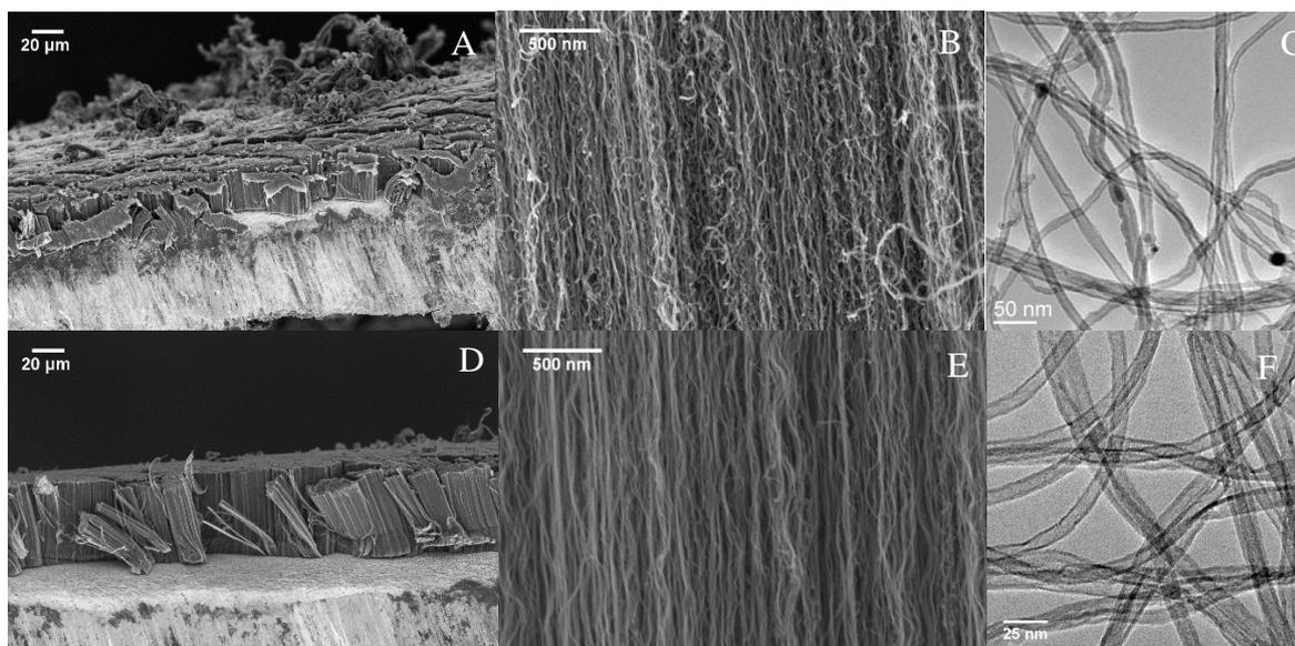
**Fig. 1.** Up: SEM (A,B) and TEM (C) images of VACNT morphology obtained on pure Al through aerosol CVD in the presence of hydrogen and acetylene; Down: SEM (D,E) and TEM (F) images of VACNT obtained with optimized synthesis parameter showing a better alignment and cleanness of the CNT.
