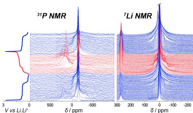
This study reports a multinuclei *in situ* NMR spectroscopic characterization of the electrochemical reactions of a  $\text{Cu}_3\text{P}$  electrode towards lithium. Taking advantage of the different nuclear spin characteristics, we have obtained real-time  $^{31}\text{P}$  and  $^7\text{Li}$  NMR data for a comprehensive understanding of the
