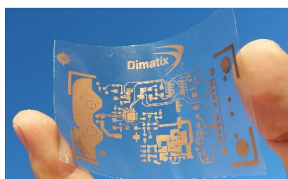
Figure 1: Copper patterns obtained on flexible substrate by electroless process after the primer printing, light-induced grafting and metallization steps.
