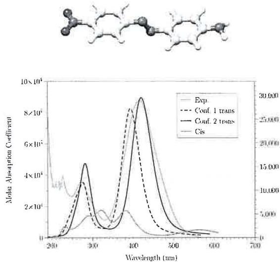
Figure 1: Disperse Orange 3 TD-DFT/CAM-B3LYP vs. experimental UV-Visible spectra
