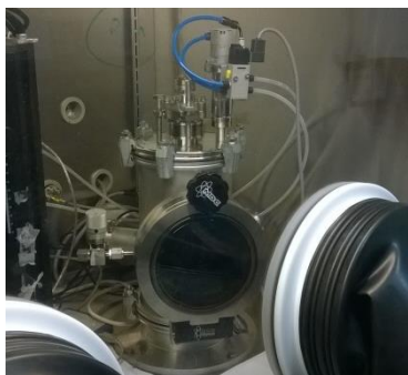
Figure a. Evaporator equipment in N 2 -filled glove box
