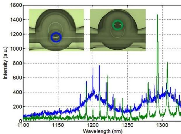
**Fig. 1. PL intensity as a function of the wavelength for two different scenarios. In blue line when the interaction region is in the coupler between ring and bus waveguide. In green line when the interaction area is placed within the ring.**
