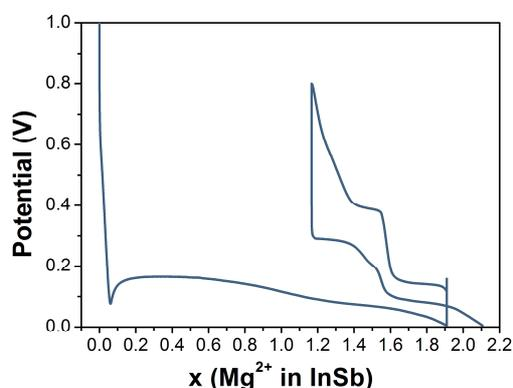
**Figure 1:** Voltage profile of an InSb-based electrode cycled at a rate of C/100 in an electrolyte based of EtMgCl and Et<sub>2</sub>AlCl in THF.
