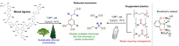
Catalytic hydrosilylation of wood lignins (left) and oxygenated plastics (right) with iridium(III) complex
