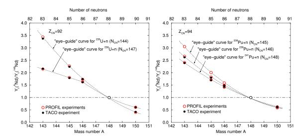
FIG. 4: Fast cumulative fission yields as a function of Nd mass number deduced from the PROFIL experiments for Uranium (left-hand plot) and Plutonium (right-hand plot) isotopes normalized to  $\overline{Y}_c(^{148}\text{Nd})$ . Our results are compared with those obtained from the interpretation of the TACO experiment [17, 18].
