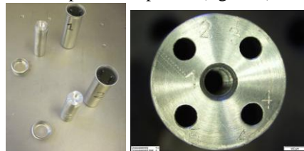
Fig.1. Left: two capsules with inner body and outside wall; right: top view of the inner body (diameter 19mm, height 60 mm) with 5 compartments.
