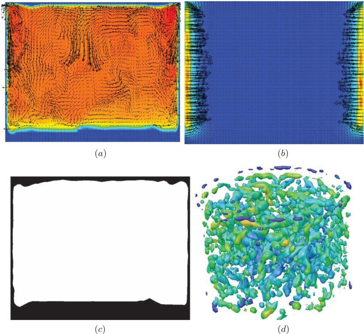
Fig. 3. Some typical results obtained after global thermal stabilization. (a) Temperature (range 2800–3277 K) and velocity vectors ( $V_{\max} = 0.03 \text{ m/s}$ ). (b) Joule power (Max:  $7662 \text{ W m}^{-3}$ ) and Lorentz forces vectors (Max:  $6400 \text{ N m}^{-3}$ ). (c) Crust profile defined by viscosity (black: solid, white: liquid). (d) Iso-contours of  $Q$ -criterion.
