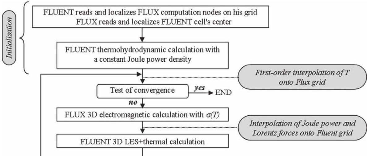
Fig. 2. Iterative algorithm for the Flux-Fluent coupling.
