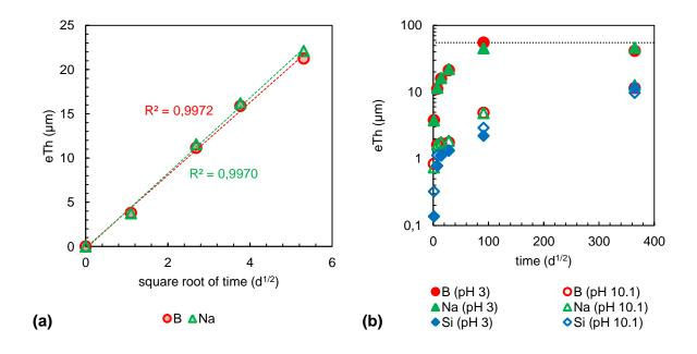
Figure 7: (a) Evolution of the equivalent thickness of altered glass, eTh, calculated from boron and sodium concentrations as a function of the square root of the time during the first month for the S1-Blk-3 test. (b) Comparison of the evolution of B, Na, and Si eTh for the S1-Blk-3 (plain symbols) and S1-Blk-10.1 (open symbols) tests. The dotted line represents the total alteration of the glass (%AG = 100).
