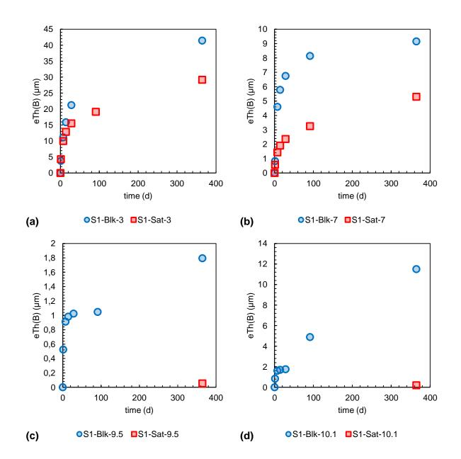
**Figure C.1:** Comparison of the evolution of the equivalent thickness of altered glass calculated from the boron concentration, eTh(B), for the S1 test series with an *S/V* ratio of 60 m<sup>-1</sup> at  $pH_{90 \, ^{\circ}C}$  values of **(a)** 3, **(b)** 7, **(c)** 9.5, and **(d)** 10.1.
