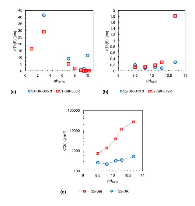
**Figure 6:** Comparison of the equivalent thickness of altered glass calculated from the boron concentrations, eTh(B), at the last sampling time ( $\approx 1$  y) at various pH for the **(a)** S1 test series (S/V = 60 m<sup>-1</sup>) and **(b)** S2 test series (S/V = 10 000 m<sup>-1</sup>). **(c)** Comparison of the silicon concentrations, *C*(Si), reached at the end of the experiment (379 d) at various pH for the S2 test series.
