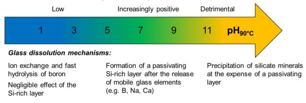
Figure 8: Diagram summarizing the effects of dissolved silica on the glass dissolution mechanisms as a function of 370 pH.
