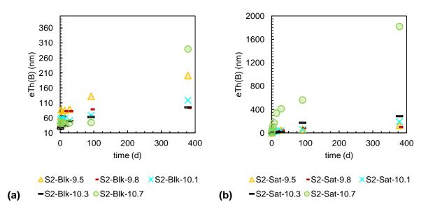
Figure 3: Evolution of the equivalent thickness of altered glass calculated from the boron concentration, eTh(B), for the (a) S2-Blk and (b) S2-Sat test series with an *S/V* ratio of 10 000 m<sup>-1</sup>. Zoomed-in subfigures are presented in Appendix B.
