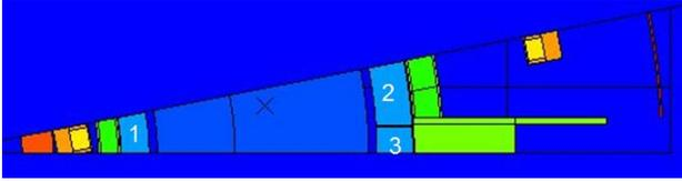
Fig. 1. Radial – toroidal cut of the DEMO 2017 half sector (11.25°); #1 inboard BB segment, #2 outboard BB lateral segment, #3 outboard central segment
