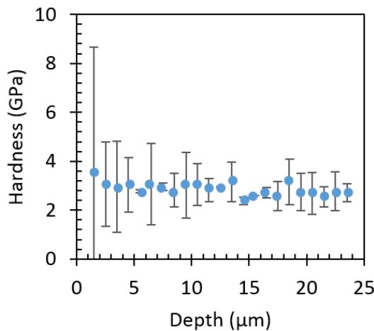
**Figure 14: Nanoindentation hardness profile of T40 sample cross section after 434 h exposure**
