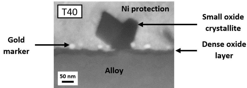
**Figure 7: SEM observation (secondary electrons) of T40 sample cross sections after 89 h exposure to primary water with preliminary gold marker deposit**
