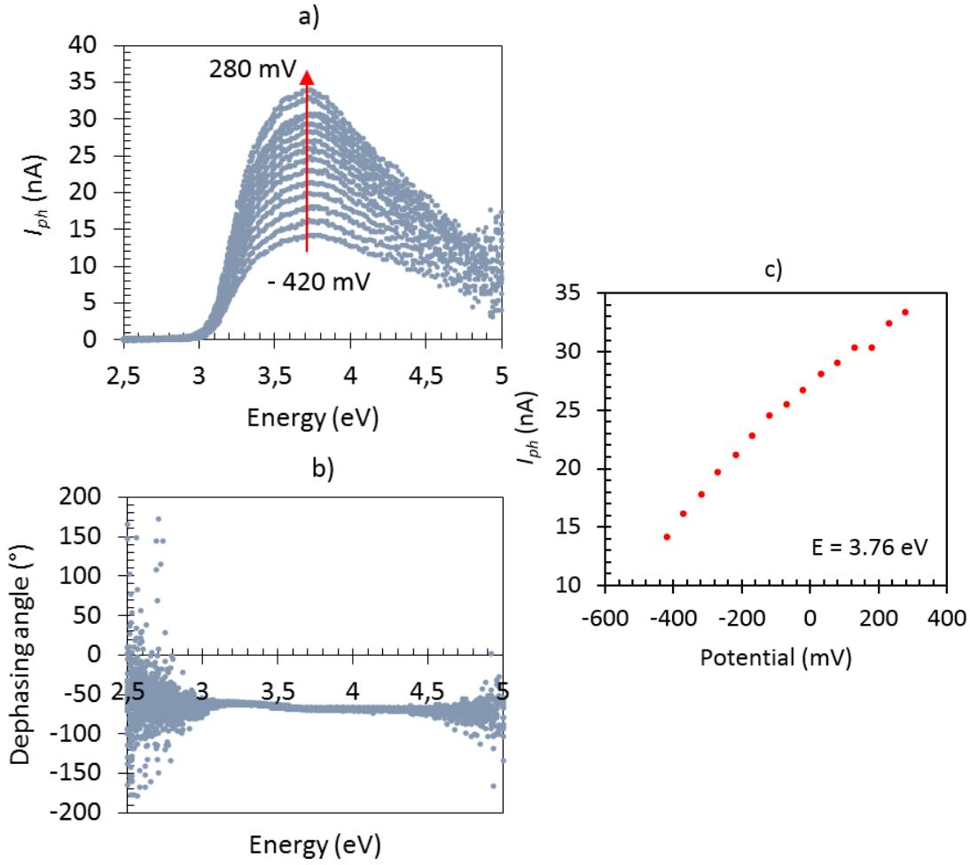
**Figure 13: a) Photocurrent ( $I_{ph}$ ) and dephasing angle ( $\phi$ ) versus incident light energy ( $E$ ) for different potential varying from -420 mV/MSE to 280 mV/MSE of T40 sample after 3499 h exposure. c) Photocurrent versus potential at 3.76 eV.**
