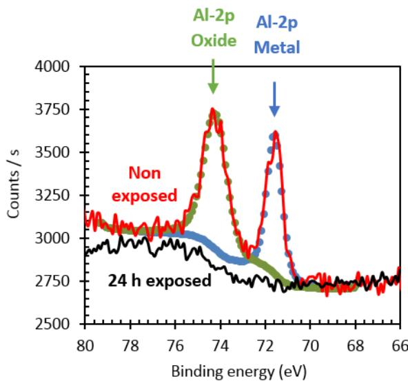
**Figure 11 : Al 2p XPS surface spectra of non-exposed and 24 h exposed TA6V samples**
