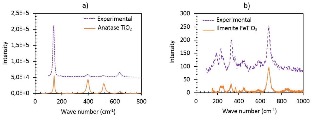
**Figure 9: Raman analysis of T40 sample surface exposed 834 h to primary water (dash lines) ; a) small crystallites and dense oxide layer and b) large crystallites ; solid lines refer to Raman spectra from reference [19] ; a)  $\text{TiO}_2$  anatase and b)  $\text{FeTiO}_3$  ilmenite.**
