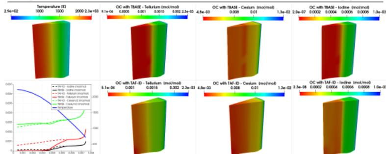
Volatile FPs release consistent with temperature profile
