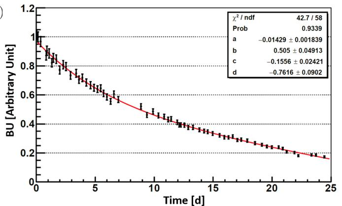
**Fig. 1.** The time evolution of the amount of fissile material in the target, so-called Burn-Up ( $BU$ ) for Exp.2. The experimental points, in black, fitted by Eq. 2, in red.
