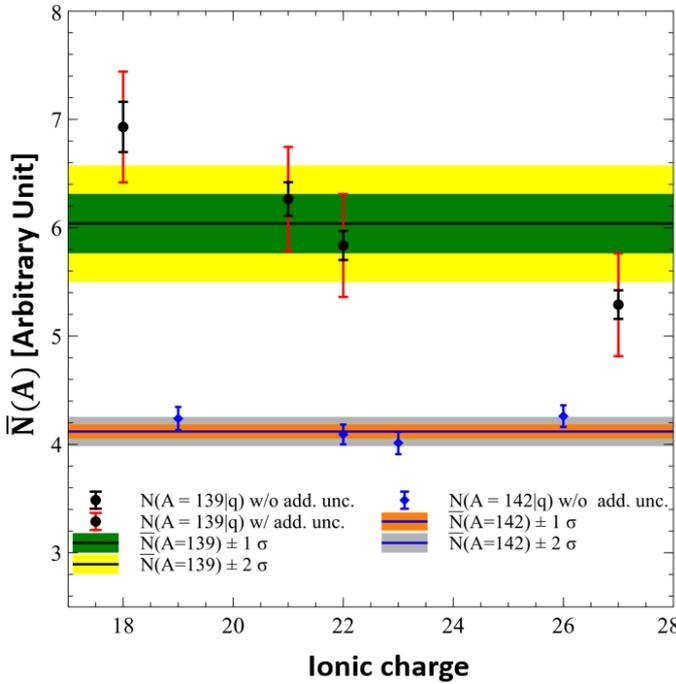
**Fig. 2.** Each  $N_{q_i}(A)$  and their mean value  $\bar{N}(A)$  for the masses 139 and 142. The compatibility criteria is met for  $A = 142$  while additional uncertainties (add. unc.) are needed for  $A = 139$ .
