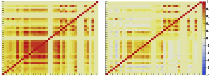
**Fig. 9.** The correlation matrix after the relative normalization when Exp.1 is the reference, on the left, and when Exp.2 is the reference, on the right. X and Y labels are identical to Fig. 12 (top).
