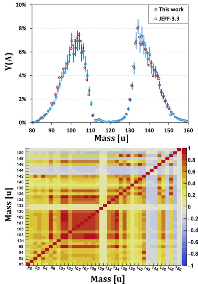
**Fig. 12.** The  $Y(A)$  for  $^{241}\text{Pu}(n_{th},f)$  and their uncertainties (at  $1\sigma$ ) obtained (in red), compared to JEFF-3.3 (in blue). On the bottom, the  $Y(A)$  experimental correlation matrix.
