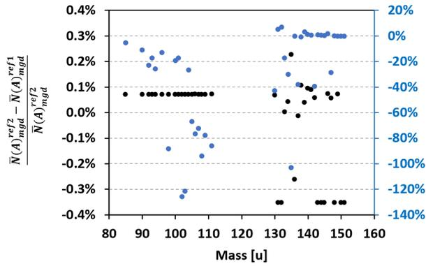
**Fig. 8.** The relative difference on  $\bar{N}(A)_{\text{mgd}}$  in black on the left axis, and on the uncertainty  $\sigma_{\text{mgd}}$  in blue on the right axis, when the reference is Exp.1 or Exp.2. For the sake of the comparison, both sets of  $\bar{N}(A)_{\text{mgd}}$  have been normalized to 1.
