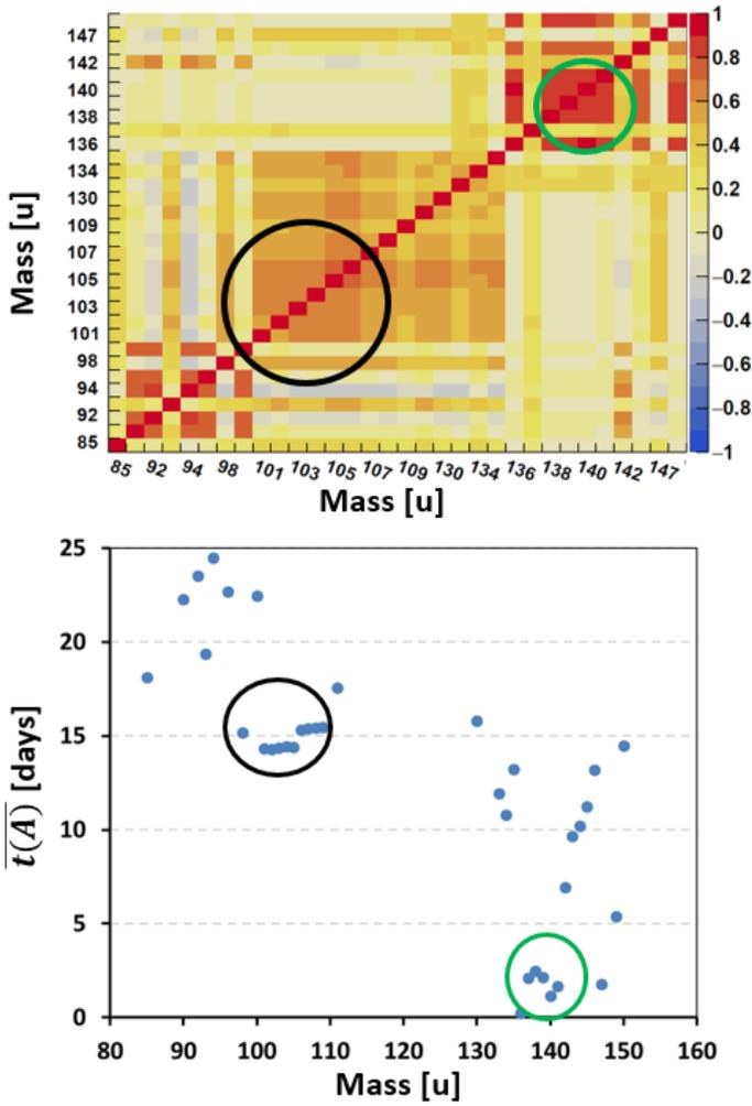
**Fig. 4.** The correlations obtained in the analysis procedure for the  $\bar{N}(A)$  for Exp.2, on the top, and the mean experimental time for each mass, on the bottom. Masses done at close experimental times (for example the masses in black or green circles) have high correlations and vice versa.
