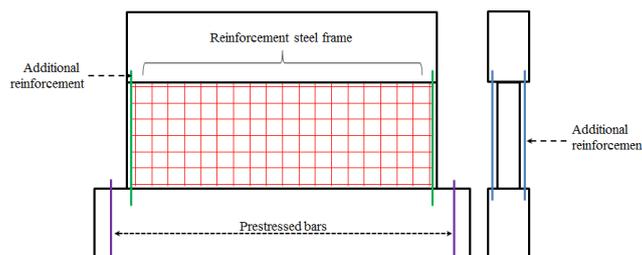
Fig. 14 Reinforcement frames for the shearing wall
