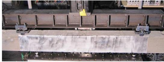
Fig. 9 Experimental device with digital image correlation
