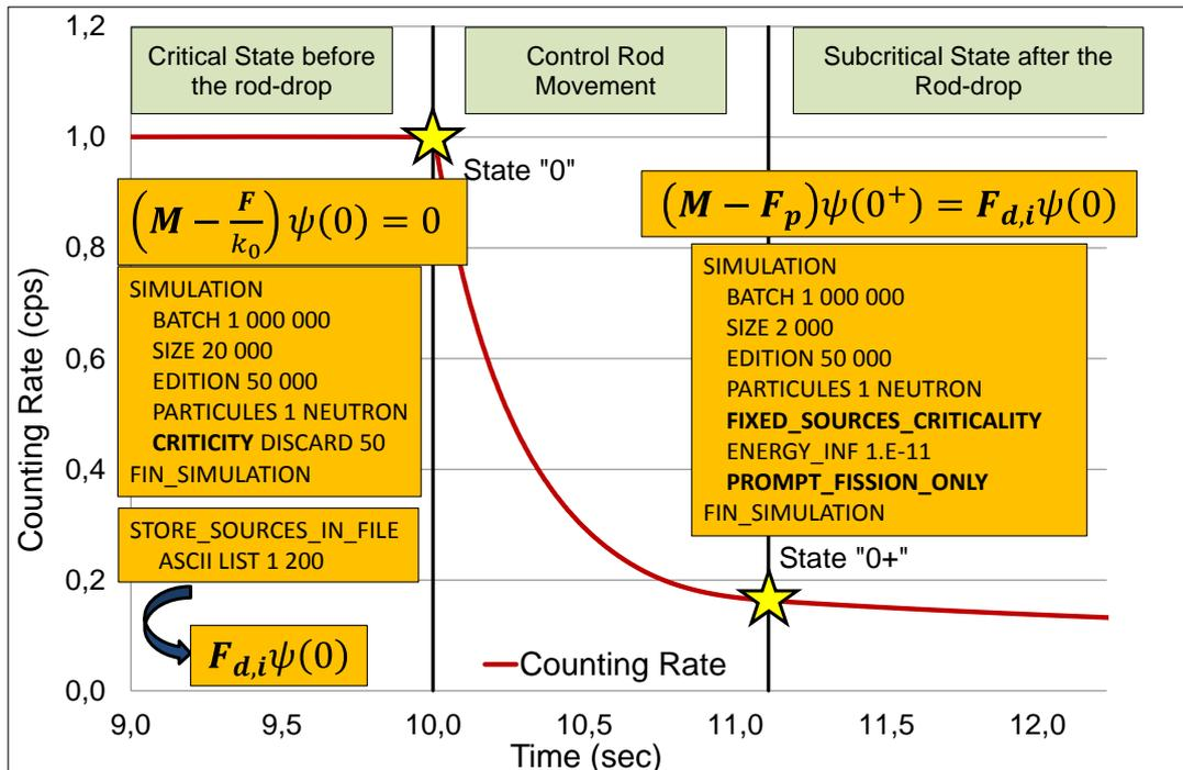
**Fig 2.** Theoretical outlet of the detector and representation of the two calculations required to interpret rod-drop experiments with a stochastic code like TRIPOLI-4®.
