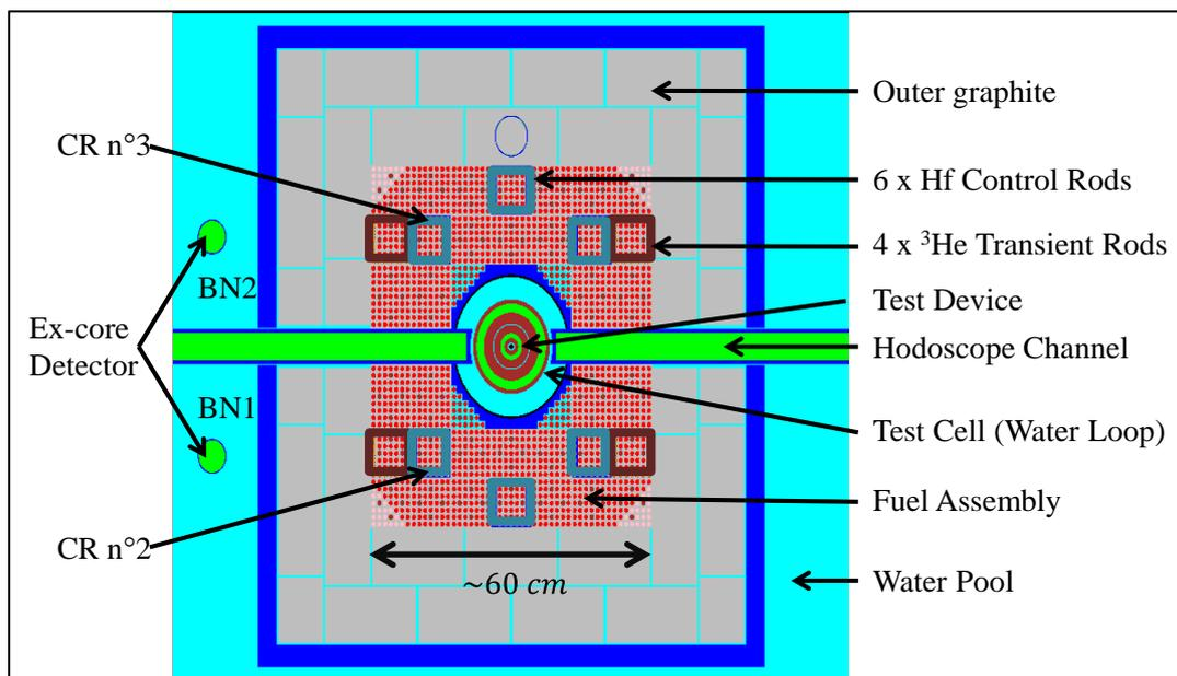
**Fig 1.** 3D Model representing the CABRI core calculated with the stochastic code TRIPOLI-4<sup>®</sup>
