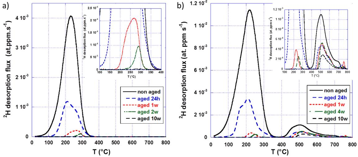
Figure 3: TDS deuterium desorption thermograms performed at  $10\text{ }^{\circ}\text{C}\cdot\text{min}^{-1}$  on a) MnAl and b) Q&P steels exposed to  $\text{D}_2$  atmosphere during their final thermal treatment (black line, just after treatment). Specimens were aged at room temperature for 24 hours, 1 week, 2 or 4 weeks, and 10 weeks and corresponding thermograms are drawn in blue, red, green and black dashed lines respectively.
