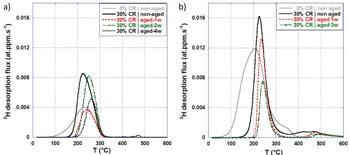
Figure 5: TDS deuterium desorption thermograms obtained on a) MnAl and b) Q&P steels exposed to  $\text{D}_2$  atmosphere during the thermal treatment (HT-specimens), before (light grey) and after (black) cold rolling (CR) up to 30 % equivalent strain, then aged (color) at room temperature during different periods of time.
