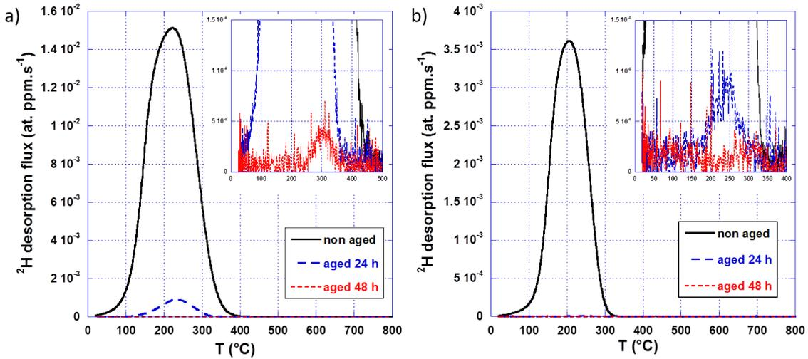
Figure 4: TDS deuterium desorption thermograms recorded on a) MnAl and b) Q&P steels treated under  $\text{N}_2$  atmosphere then cathodically charged for 1 hour at  $80\text{ }^{\circ}\text{C}$  in  $0.1\text{M NaOD}$  solution. The thermograms obtained just after deuterium charging are in black; those obtained after 24 h and 48 h duration room temperature aging are in blue and red, respectively.
