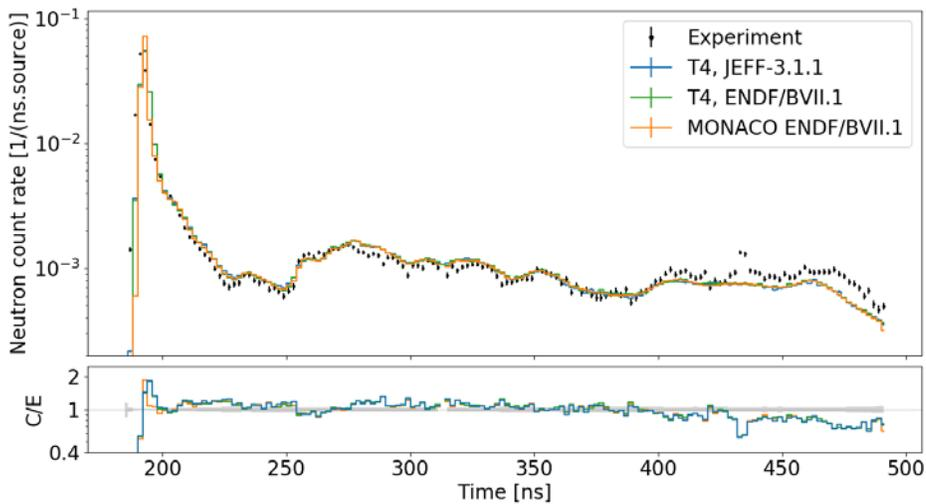
**Fig. 13.** Neutron counts at  $120^\circ$  with concrete sphere.
