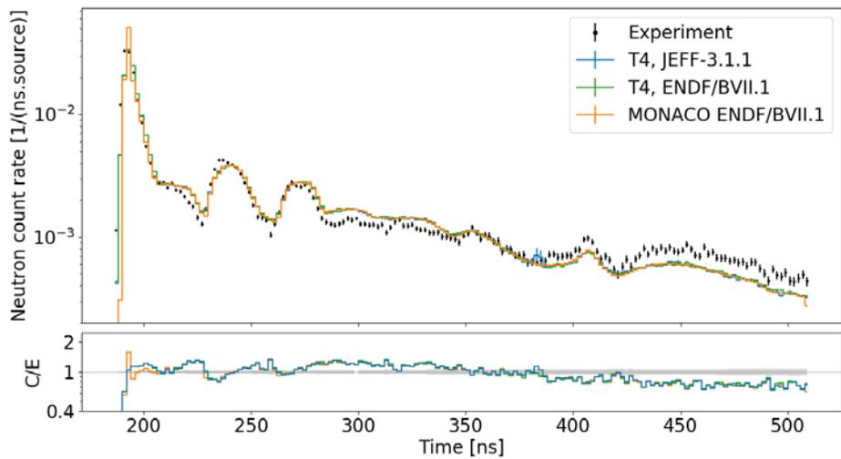
**Fig. 6b.** Neutron counts at 120° with C sphere.
