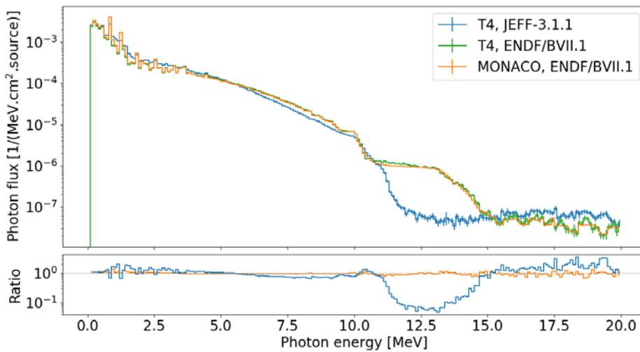
**Fig. 11.** Gamma flux on surface of iron sphere.
