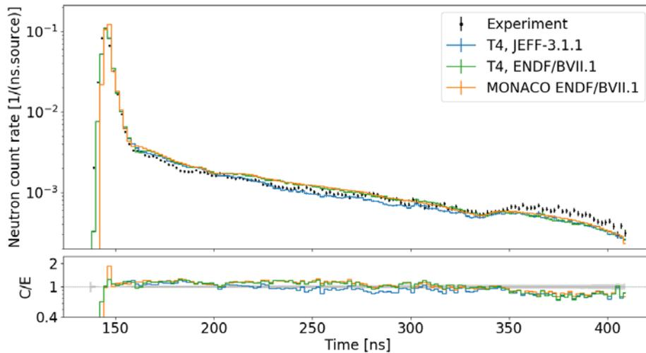
Fig. 4. Neutron counts at 30° with Be sphere.
