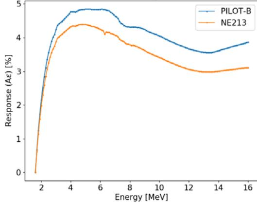
**Fig. 3.** Pilot B and NE213 detector response functions.
