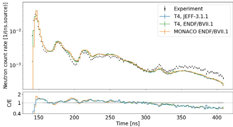
**Fig. 6a.** Neutron counts at 30° with C sphere.
