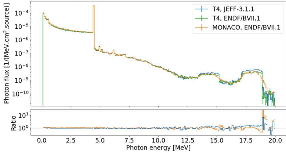
**Fig. 7.** Gamma flux on surface of C sphere.
