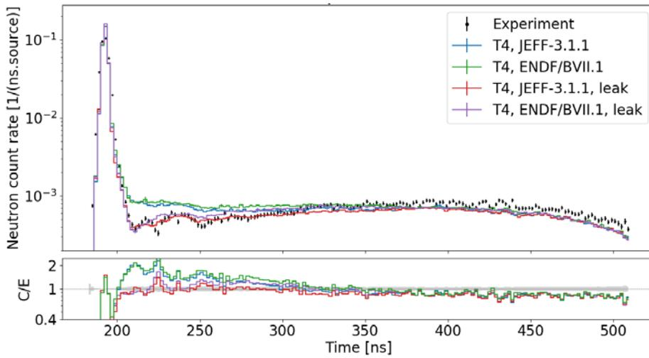
**Fig. 12b.** Neutron counts at  $120^\circ$  with iron sphere – no collimator contribution.
