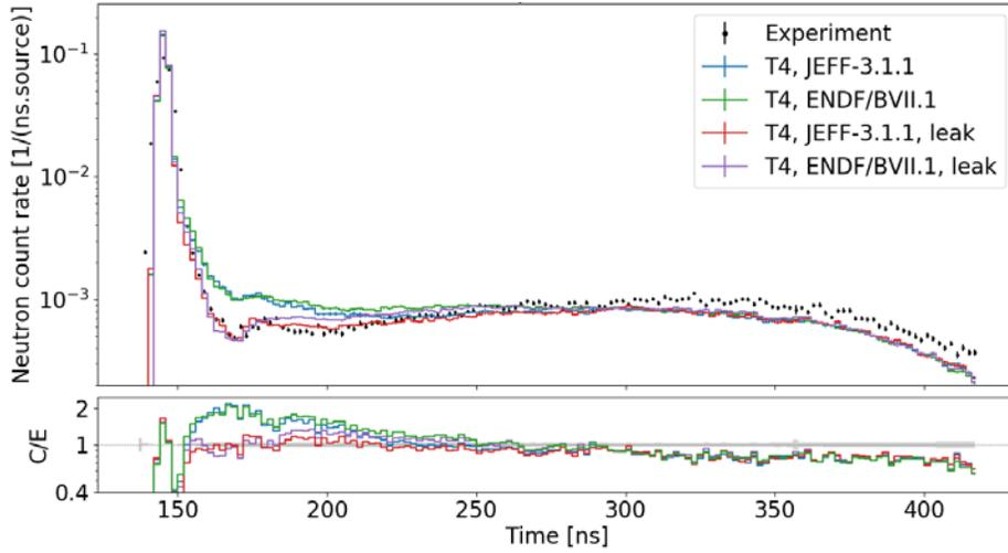
**Fig. 12a.** Neutron counts at  $30^\circ$  with iron sphere – no collimator contribution.
