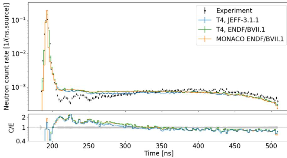
**Fig. 10b.** Neutron counts at 120° with iron sphere.
