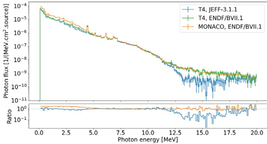
**Fig. 5.** Gamma flux on surface of Be sphere.
