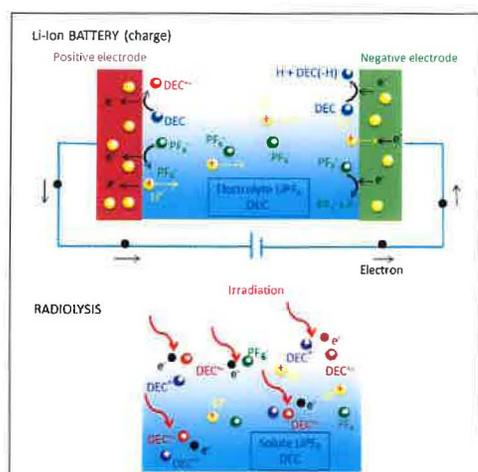
Fig. 1. Scheme comparing primary electron transfers at the electrodes in the electrolytic charge/ageing processes of a Li-ion battery (with molar DEC/ LiPF<sub>6</sub> solution as a model electrolyte) (top), and after ionization in the bulk in the radiolytic process with the same medium (bottom).
