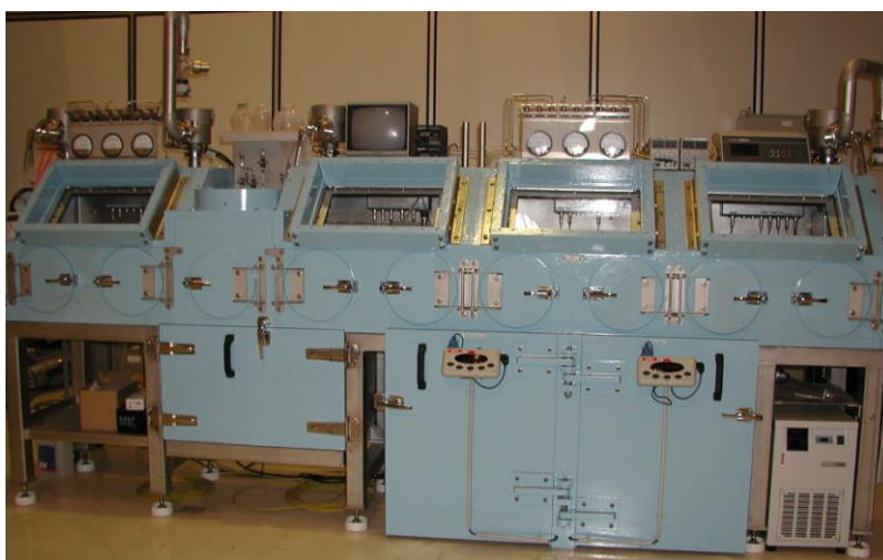
Figure 4. The glove box for the electropolishing machine
