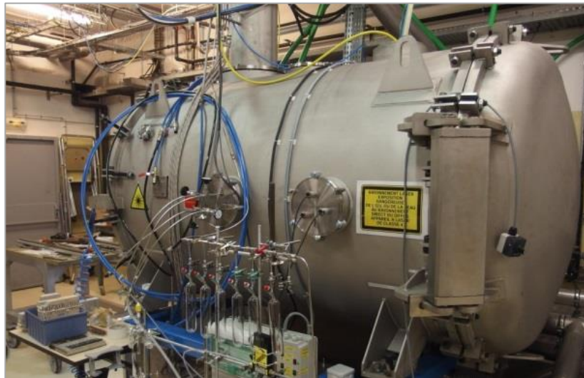
Figure 2. View of the cutting cell of the DELIA facility
