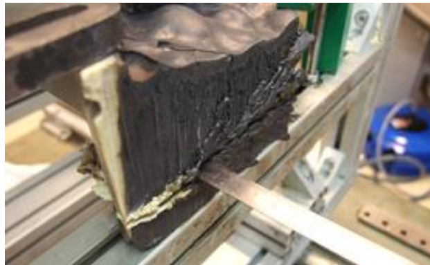
Figure 3. View of laser-cut fuel debris simulant for ex-vessel configuration
