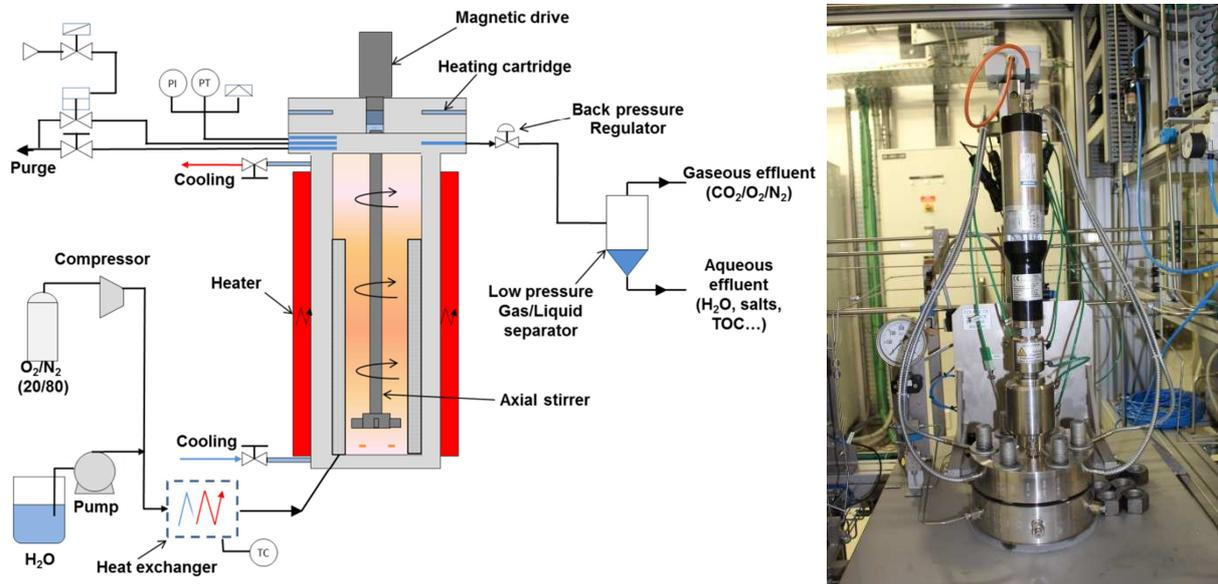
Figure 3: Overall Flowsheet of SCWO dynamic batch reactor
