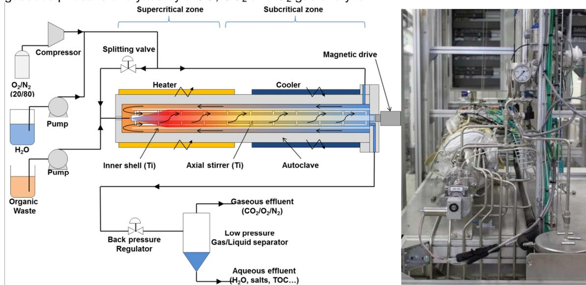
Figure 1: Overall flowsheet of SCWO 200 g.h<sup>-1</sup> process
