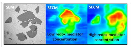
**Fig. 1**: Presentation of the combined SEM-SECM responses at the basis of an advanced electronic transport characterization. Taken from 3
