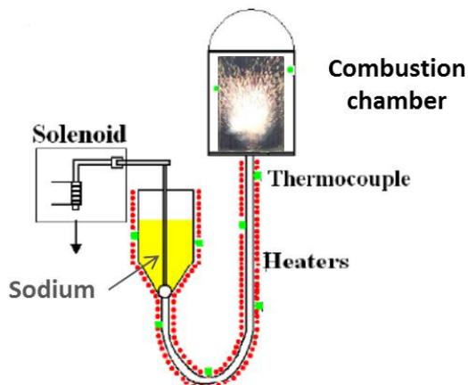
Figure 5: Basic principle of spray fire demonstrative facility
