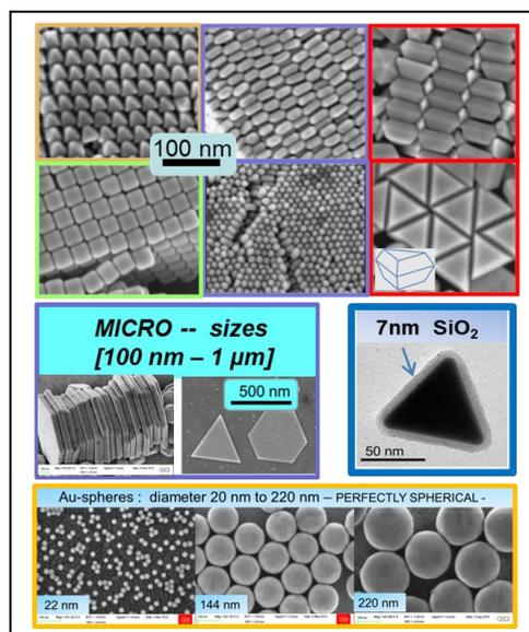
**Figure 1:** Illustration of some of our monodisperse gold nano-particles, micro-plates and hybrids (Au@SiO<sub>2</sub>) with tunable sizes and thicknesses.
