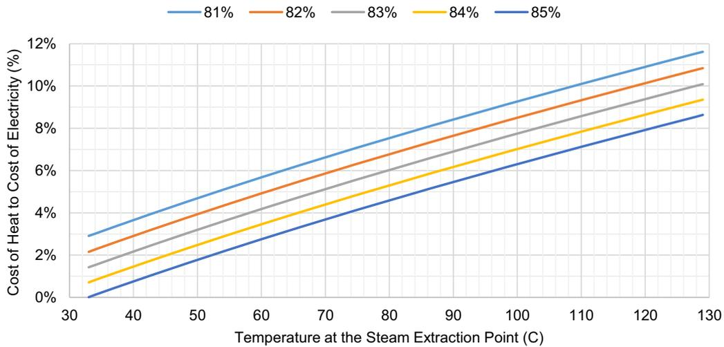
Fig. 10. Cost of heat to cost of electricity vs. temperature at the steam extraction point (Method 2) for different values of (DPP<sub>2</sub>) availability.
