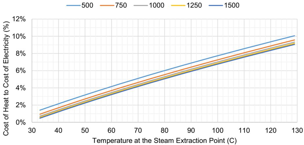
Fig. 9. Cost of heat to cost of electricity vs. temperature at the steam extraction point (Method 2) for different values of process thermal power (MW<sub>th</sub>).
